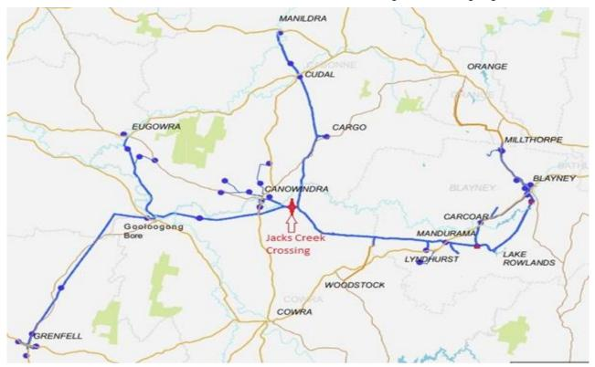
The location of the break was between Trunk Main "V" the main feed to the Moorbel Reservoir that supplies the Canowindra township and Trunk Main "U", the supply to Canomodine Pump Station which services Cargo, Cudal and Manildra townships.
